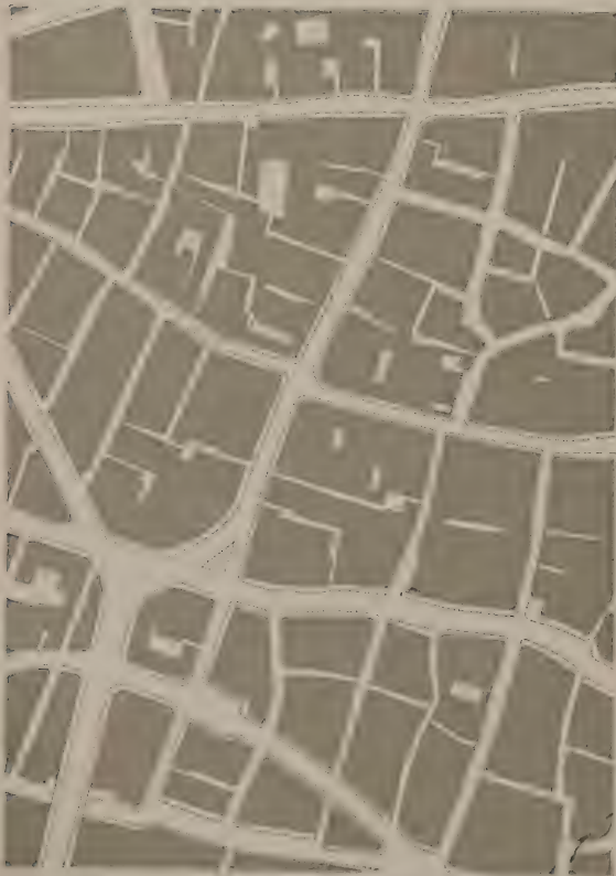
50 The inherited urban road pattern—irregular alignments, narrow streets, frequent intersections.
